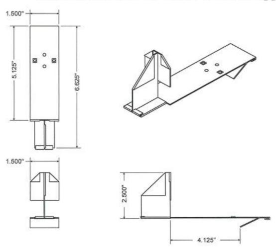
MATERIAL: Our model No.-4 Snow-Guard is manufactured using .020 thickness of cold rolled copper. Since it is double thick the result is  $.020 \times 2 = .040$ .
